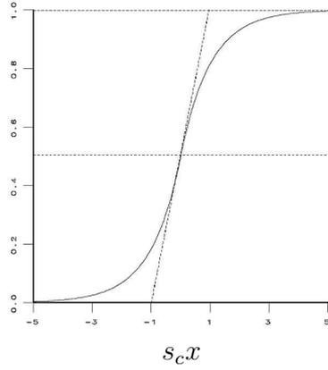
Fig. 1. Edge model defined as an exponential function with  $s_c > 0$
