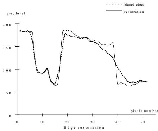
Fig. 9. Image cross section: blur edge profile and its restoration.
