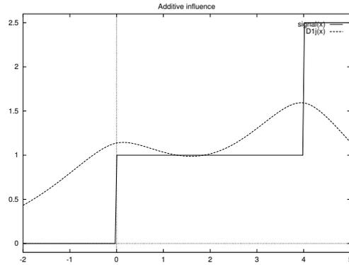
Fig. 4. Additive influence of a neighbor edge: the detection amplitude increases and the highest response maximum moves toward the coarse scales as the detector scale decreases.
