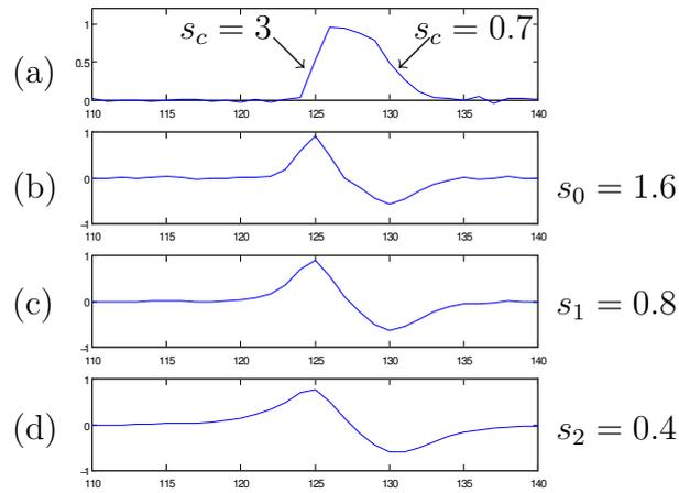
Fig. 5. (a) Edge profiles ( $s_c = 3$  and  $s_c = 0.7$ ) and (b), (c), (d) multiscale analysis ( $s_0 = 1.6, s_1 = 0.8, s_2 = 0.4$ ). The best detection is achieved by the first scale for " $s_c = 3$ " profile while the second scale performs the best detection for " $s_c = 0.7$ " profile.
