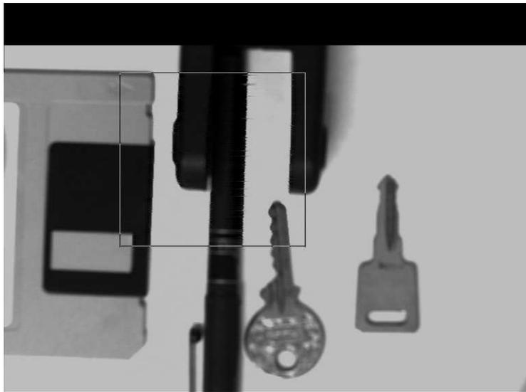
Fig. 15. Restoration by an autonomous system: camera ( $740 \times 580$  pixels) and DSP (ADSP 2181 - 40MHz). This figure shows the blurred image and a piece ( $256 \times 256$  pixels) of restoration (inside the square outline).
