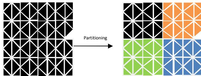
Figure 3 : example of our mesh partitioning in 2D.
