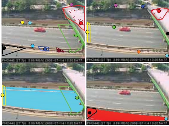
Figure 5. Results from our clustering method. Top left: 9 entry areas, top right: 8 exit area. Bottom left and right, MPs with the largest number of tracks together with their entry and exit areas.
