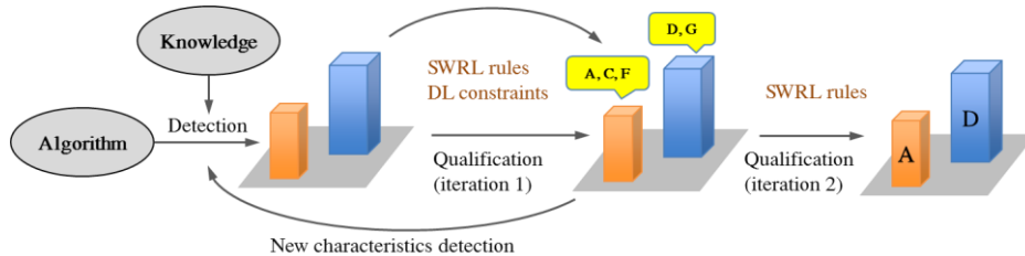
Fig. 5: Knowledge driven method for object detection and qualification process.
