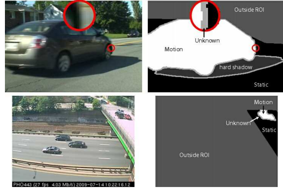
Figure 2. Sample frames showing 5-class ground-truth label fields.
