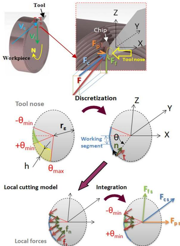
Fig. 3. Modeling local forces in face turning
