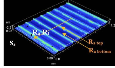
Fig. 2. Directions of roughness measurement (in 3D cutting)
