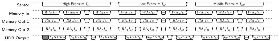
Figure 3. Memory Management Core. Performing three parallel streaming videos with low ( $I_L$ ), middle ( $I_M$ ) and high ( $I_H$ ) exposure times. The delayed HDR row output is shown after HDR and tone mapping computations (related to Section 3.3 and 3.4.
