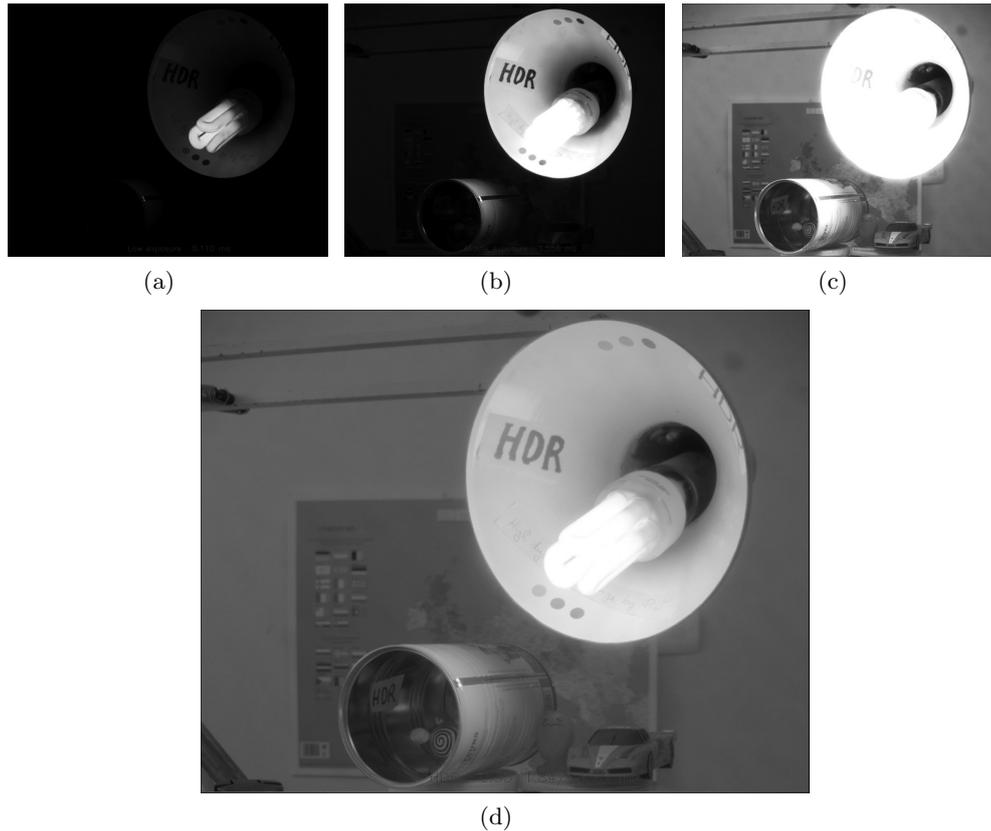
Figure 5. Result of the complete system. Our Multiple Exposure Control can select the three proper exposures, and the specific memory management core permits us to display 3 bracketed images at the same time.
