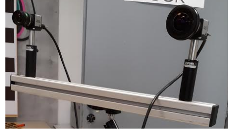
Fig. 3 Hybrid stereo-vision rig used for our evaluation
