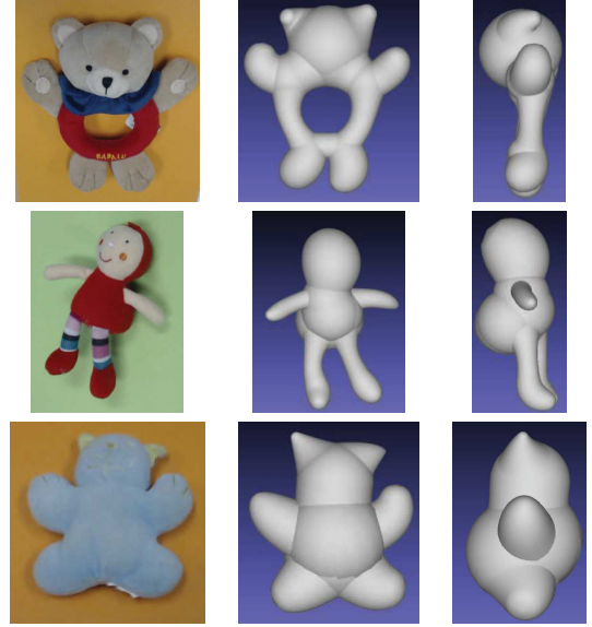
Figure 7. Reconstruction of different objects using the proposed method. Left column: one of the two input images. Middle, right columns: front and side views of the reconstruction. Tubular parts like arms are well reconstructed, whereas flat parts like the body of the third object are not, giving a rounded shape to the objects.
