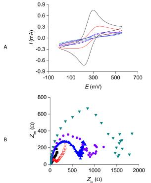
**Figure 2.** Characterization of Au/SAM/L bilayer by EIS. Cyclic voltammograms (A) and Nyquist plots (B) of the  $[Fe(CN)_6]^{3-}/[Fe(CN)_6]^{4-}$  redox couple (1 mM each in 0.5 M KCl) recorded for a bare gold surface (black), octanethiol Au/SAM (2 min exposure in 1 mM ethanol solution of octanethiol; red), Au/SAM/LB(L) (blue), and Au/SAM/LB(C) electrodes (3 min exposure of Au/SAM/LB(L) to  $10^{-11}$  M (violet) and  $10^{-6}$  M (green) aqueous solution of Hg(ClO<sub>4</sub>)<sub>2</sub>).
