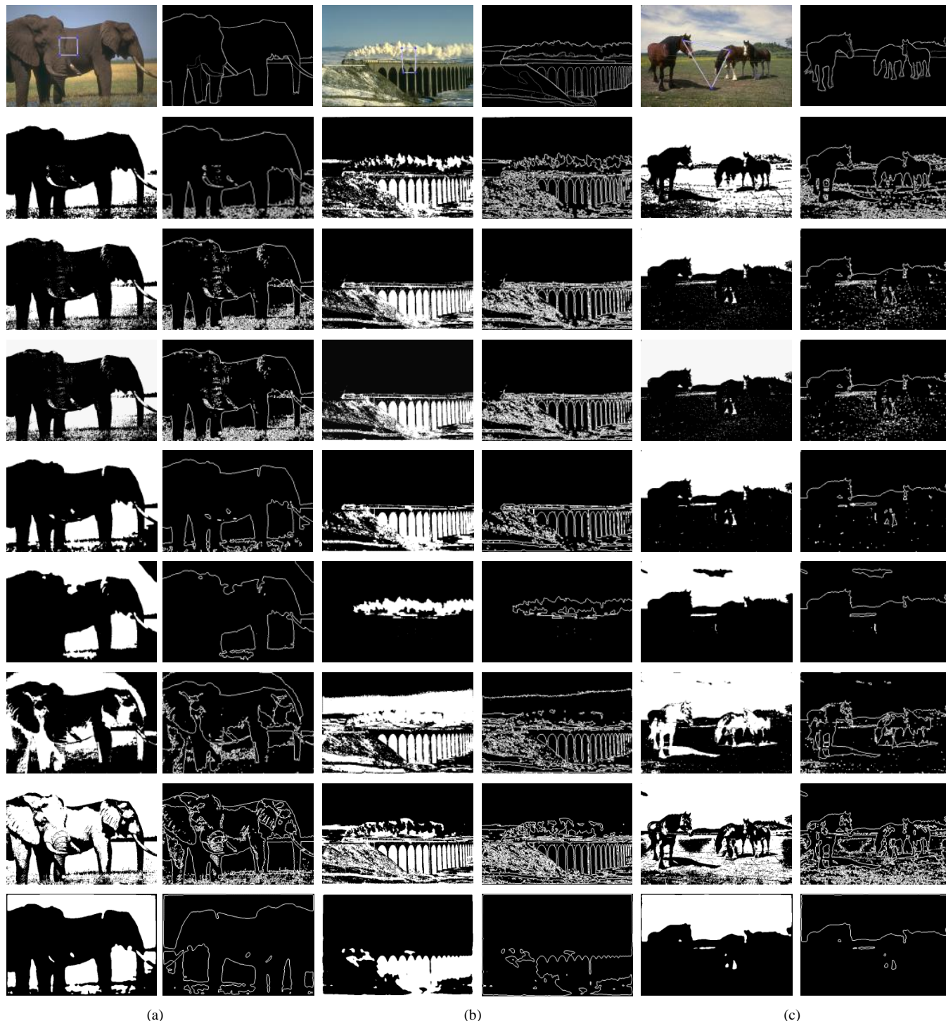
Fig. 6. Segmentation of real-world images. The first row presents the original images with the initial contour, and the corresponding human segmentation as ground truth. The second row presents the results of the proposed algorithm. The third row presents the results of the k-means clustering method. The fourth row presents the results of the FCM clustering method. The fifth row presents the results of the PKGC method. The sixth row presents the results of the CV method. The seventh row presents the results of the HZ method. The eighth row presents the results of the Li method. The last row presents the results of the GF method. For all the methods, the results are presented in two ways, i.e., by contours and binary images.
