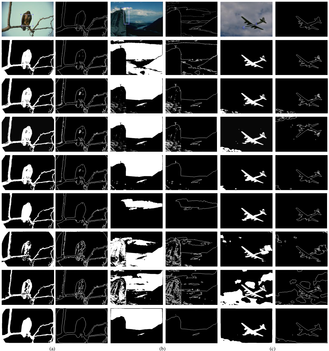
Fig. 7. Segmentation of real-world images. The first row presents the original images with the initial contour, and the corresponding human segmentation as ground truth. The second row presents the results of the proposed algorithm. The third row presents the results of the k-means clustering method. The fourth row presents the results of the FCM clustering method. The fifth row presents the results of the PKGC method. The sixth row presents the results of the CV method. The seventh row presents the results of the HZ method. The eighth row presents the results of the Li method. The last row presents the results of the GF method. For all the methods, the results are presented in two ways, i.e., by contours and binary images.
