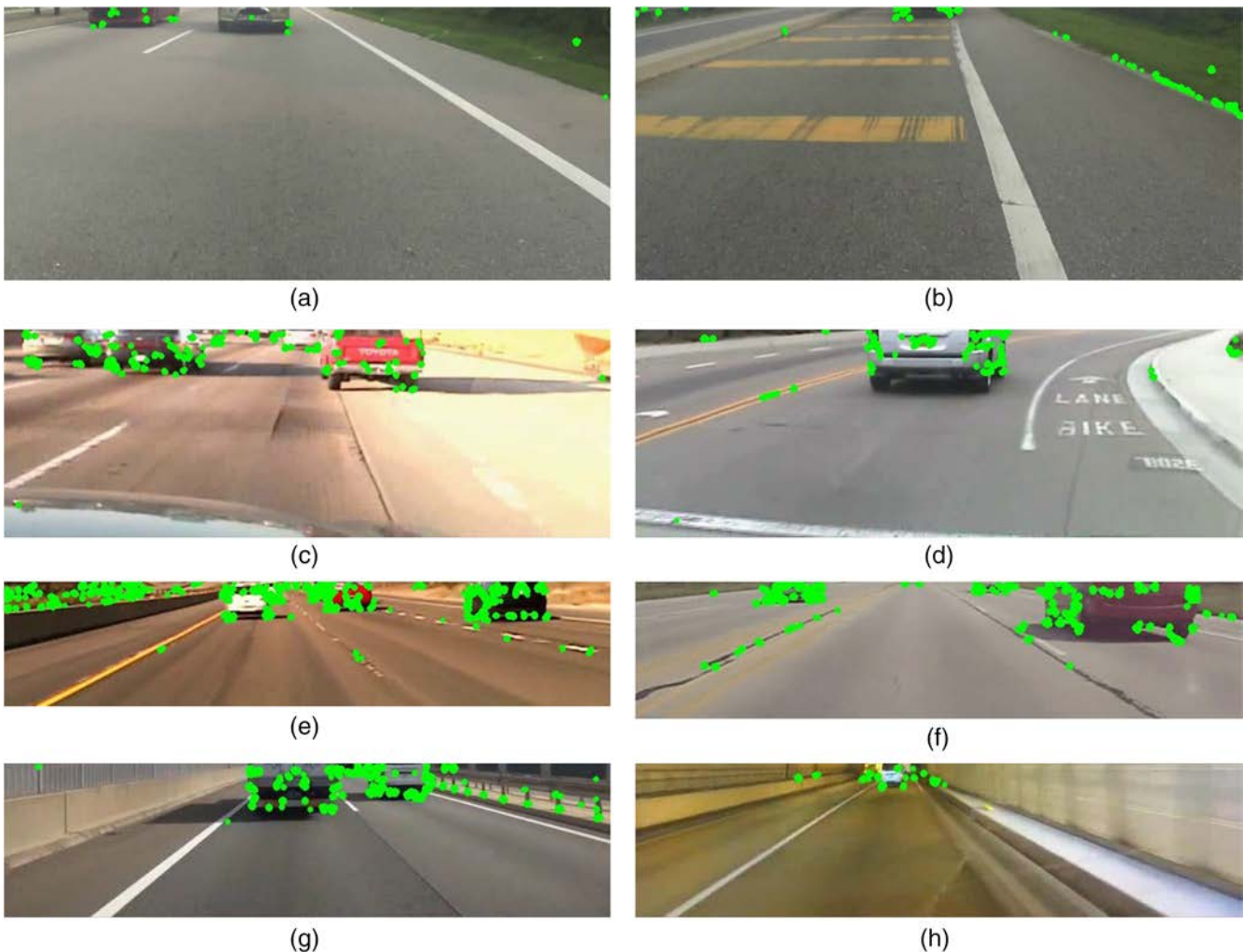
Fig. 9 Harris corner detection: (a) incoming vehicles from self-recorded dataset, (b) truck from self-recorded dataset, (c) LISA-dense (frame 735), (d) LISA-urban (frame 13), (e) LISA-sunny (frame 104), (f) source-2 (frame 140), (g) iROADS-daylight, and (h) iROADS-tunnel.
