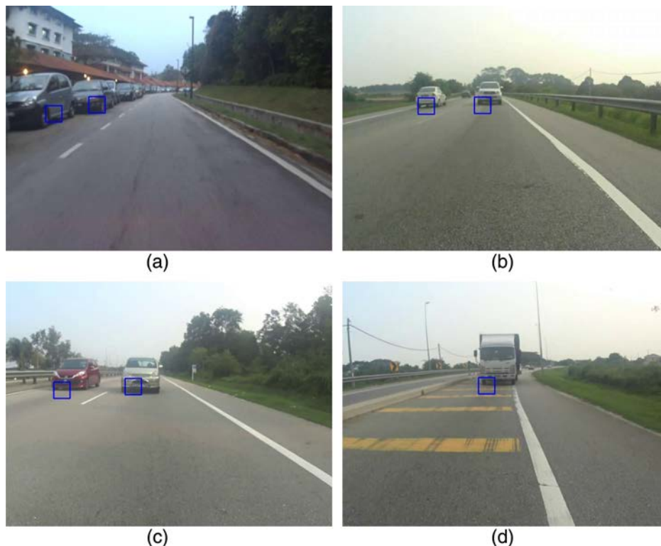
Fig. 11 Vehicle detection from self-recorded dataset: (a) vehicles are parked on the roadside, (b) moving vehicle in a single lane, (c) vehicle detection on a road with multiple lanes, and (d) truck detection at lane markers.
