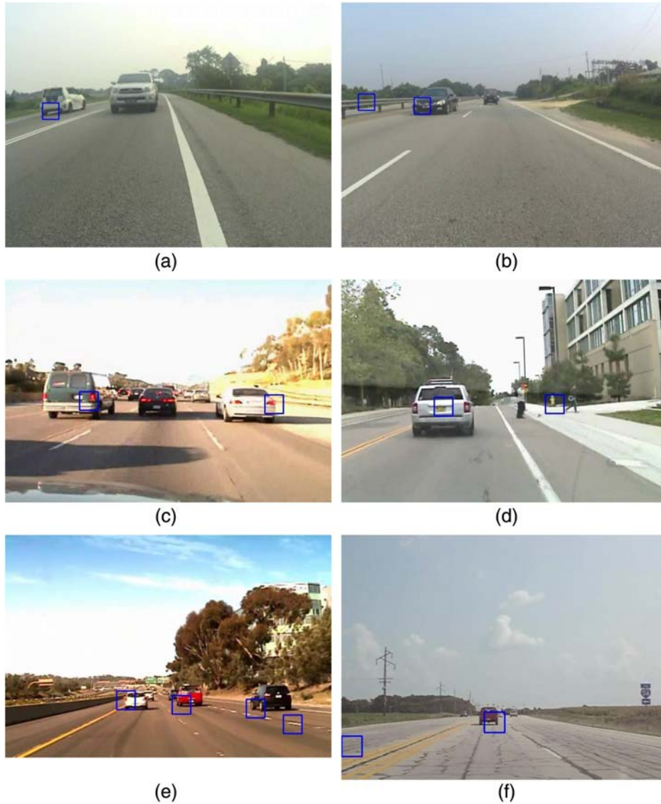
Fig. 13 False vehicle detection: (a) missing vehicle detection in self-recorded dataset, (b) false detection from self-recorded dataset, (c) LISA-dense (frame 735), (d) LISA-urban (frame 13), (e) LISA-sunny (frame 104), and (f) source-2 (frame 744).
