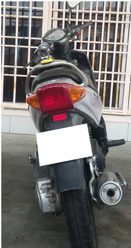
Fig. 1 Sony action cam mounted at the rear end of motorcycle.
