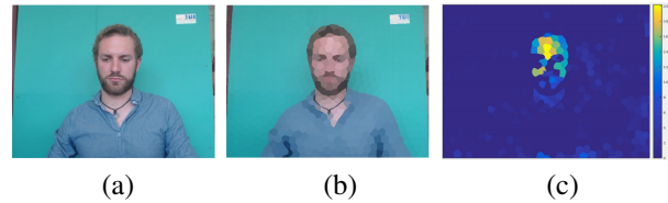
Fig. 1. Pulsatility measures estimated from various temporal superpixels. (a) input frame, (b) temporal superpixel segmentation and (c) pulsatility measures (blue means low pulsatility measures and yellow/orange is high).
