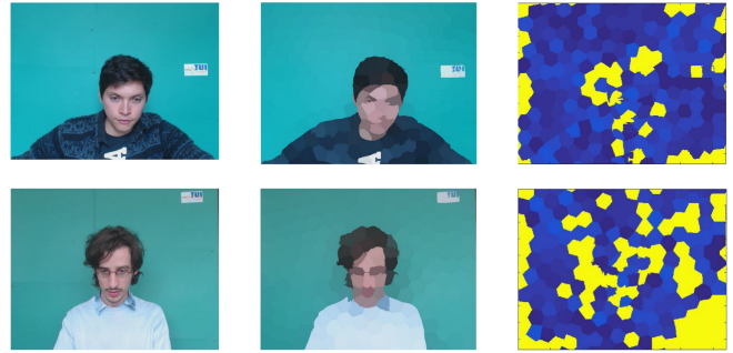
Fig. 11. TSP tracking failure examples. The second column shows the TSP segmentation while the third column highlights in yellow the tracking failures.
