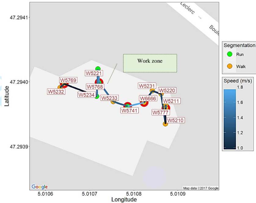
Figure 12. Visualizing a complete worker` trajectory with semantic stay points in red colored circles (site identifications for e.g. W5768 for a workzone), semantic lines (segmentation into run and walk points) and a semantic region
