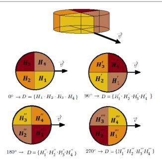
Fig. 19 Descriptor construction relative to the frontal orientation vector  $\overrightarrow{v}$ : (top) cylinder division into blocks; (down) each rotation of the frontal vector yields a new descriptor.
