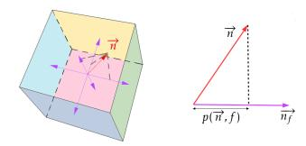
**Fig. 9** Quantization of the normal vector  $(\overrightarrow{n_i})$  using a cube  $(n_s=6)$ : a)  $\overrightarrow{n_i}$  is positioned at the center of the polyhedron to be projected on each vector  $\overrightarrow{g_s}$  that connects the center of the polyhedron and the center of its face s. b) the projection of  $\overrightarrow{n_i}$  on the vector  $\overrightarrow{g_s}$ , the result is the scalar value  $\widehat{q}_{i,s}$ .
