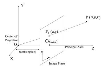
Fig. 4 Illustration of the pin-hole camera model.
