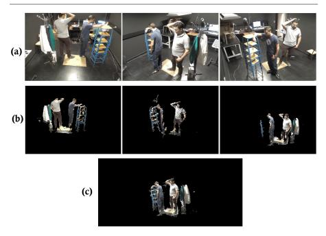
Fig. 21 Data obtained for each scene: a) RGB images b) Single Point Cloud (SPC) from each kinect, c) CPC of the scene.
