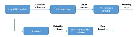
Fig. 11 Human detection procedure pipeline.
