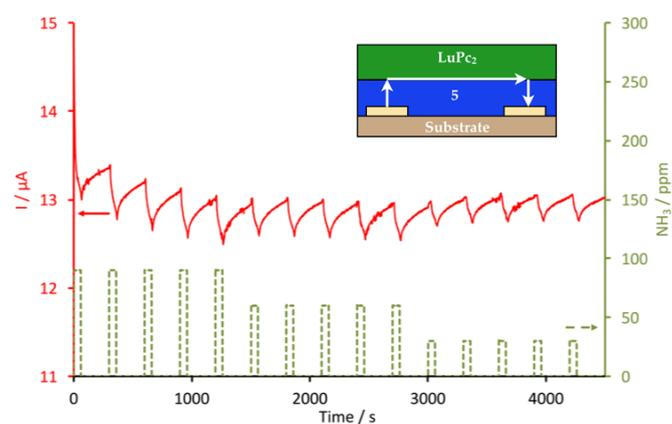
**Fig. 6** Response of a **5**/ $\text{LuPc}_2$  MSDI heterojunction to ammonia ( $\text{NH}_3$ , 90, 60 and 30 ppm), at 30% relative humidity, during exposure/recovery cycles (1 min/4 min).
