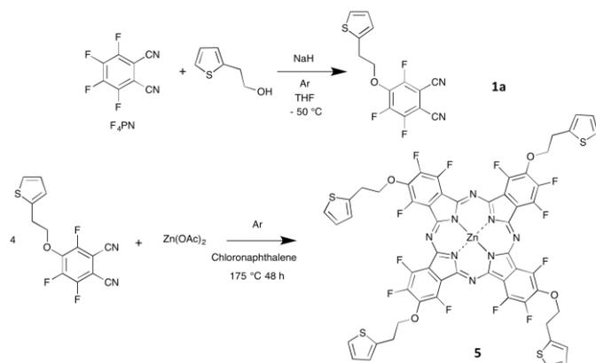
**Scheme 1** Synthesis of the phthalocyanine **5** (the isomer  $C_{4h}$  is shown) and its precursor **1a**
