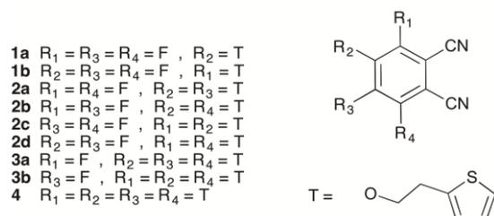
**Scheme 2** List of all the phthalonitrile derivatives identified during the reactions of 2-(2-thienyl)ethanol with tetrafluorophthalonitrile
