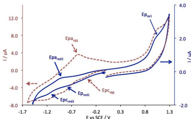
**Fig. 3** CV of **5**, on Pt disc electrode, in DMF containing 0.1 M Bu<sub>4</sub>NPF<sub>6</sub>, at a scan rate of 0.1 V s<sup>-1</sup>, at a concentration of 10<sup>-3</sup> mol L<sup>-1</sup> (solid blue line) and at 4x10<sup>-3</sup> mol L<sup>-1</sup> (aggregation, dashed red line).
