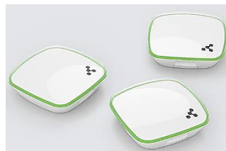
Fig. 1. BLE beacons by Kontakt.io used to collect spatio-temporal data
