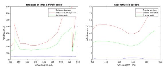
**(b)** Raw data obtained from the pixels of the **(c)** Corresponding estimated spectra. multispectral image.
