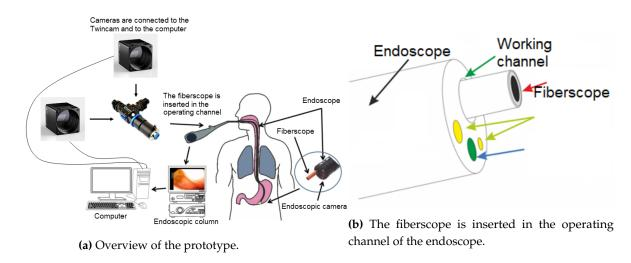
Figure 2. Functional scheme of the prototype.
