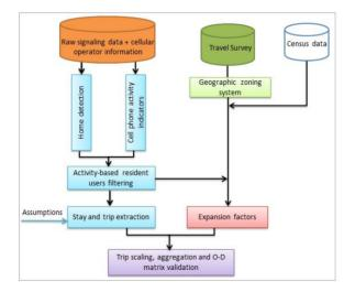
Fig. 2 Workflow of Origin-Destination matrix construction from cellular network signalling data
