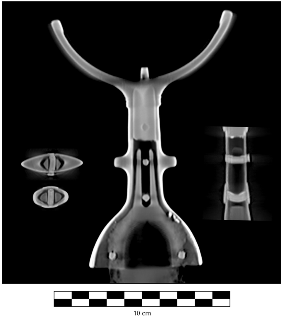
Figure 3: Different cuts on the 3D model resulting from the CT-scan depicting the organisation of the hilt, the blade tang and the rivets. © BCRX and T. Nicolas.
