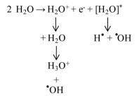
Figure 2. Production of oxygen free radicals during radiolysis.
