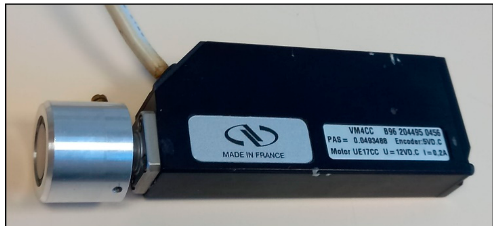
Figure 15. Actuator of the push force control system by Micro-Contrôle Corp.
