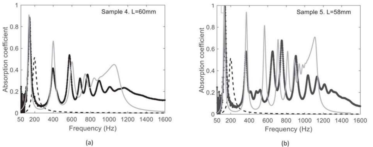
Figure 2: Absorption coefficient experimental data (black markers) and model predictions (grey lines) for hard backed absorbers composed of 1 mm thick plates with spacings between the plates of (a)  $d_c = 1 \text{ mm}$  and (b)  $d_c = 3 \text{ mm}$ . Predictions for Helmholtz resonator of same size as the absorber (dashed lines).
