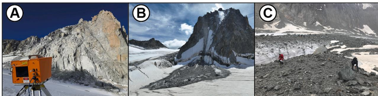
Fig. 2. Used methods. (A) Example of TLS survey on the east face of Tour Ronde. (B) Example of a rockfall in the north face of Tour Ronde documented by the network of observers (August 2022,  $12 \times 10^3$  m<sup>3</sup>). (C) Sampling of clasts on supraglacial moraines for <sup>10</sup>Be concentration analysis.
